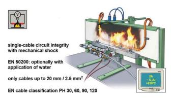
Figure 2: Testing a single cable in accordance with DIN VDE 0882-200 (previously: DIN VDE 0472-814), EN 50200, IEC 60331-25
